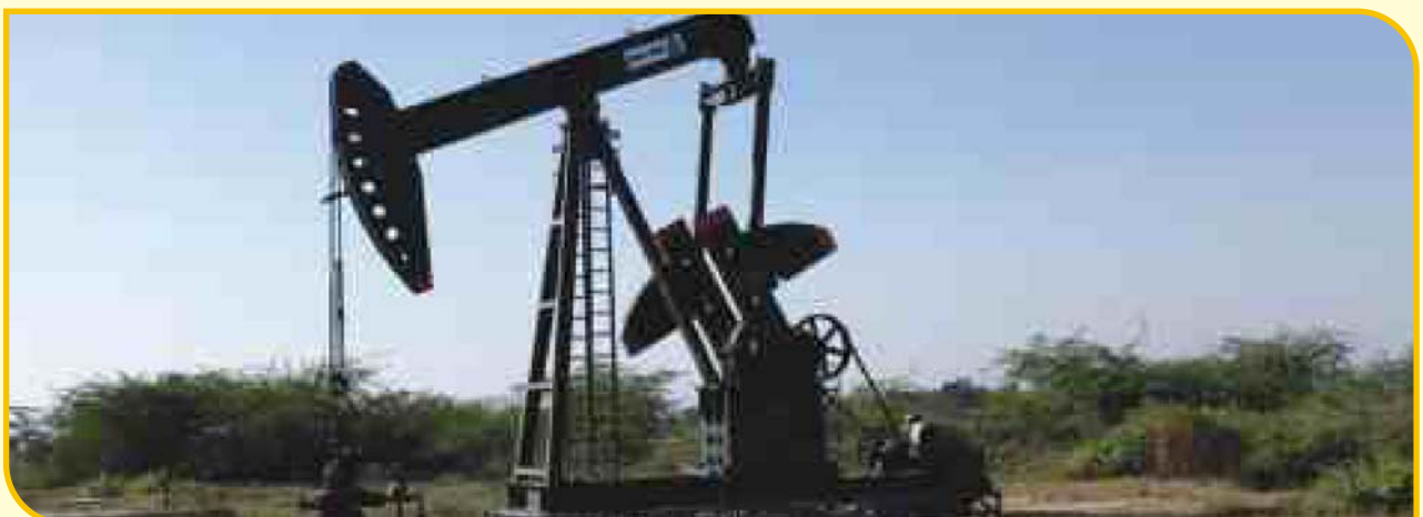
Sucker Rod Pump : Mainstay in brownfield production
